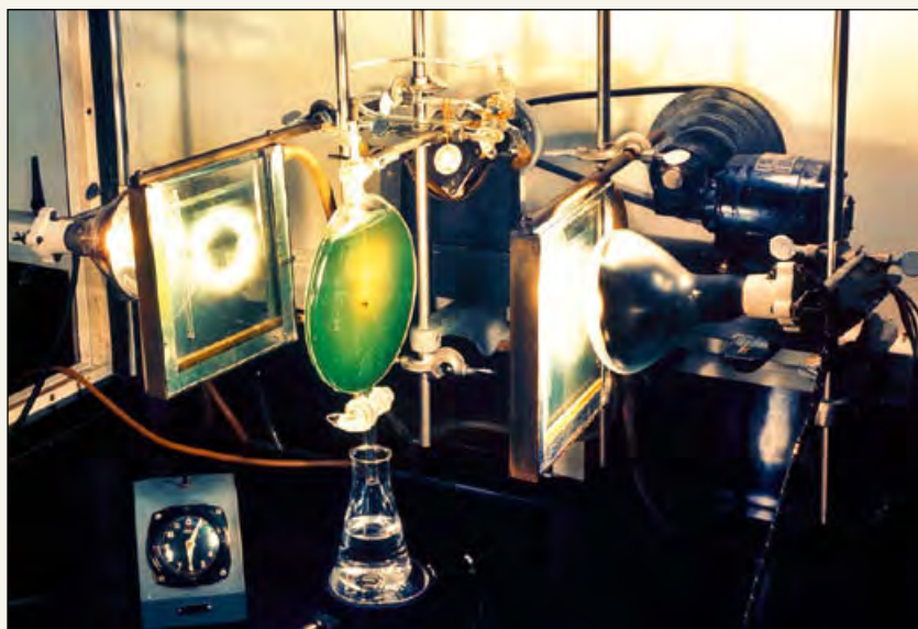
Figure 8.21 Calvin's apparatus for investigating the light-independent reactions of photosynthesis.
