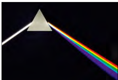
Figure 2.33 ‘White light’, such as sunlight, is composed of a range of wavelengths, which become separated as they pass through a glass prism.
